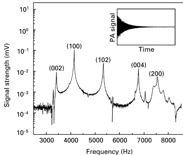
**Figure 7** Time-dependent PA signal recorded by a microphone (inset) and corresponding frequency spectrum of a cylindrical resonator. In the displayed frequency range, the second longitudinal (002), first radial (100), combination (102), fourth longitudinal (004) and second radial (200) modes of the resonator are detected.
