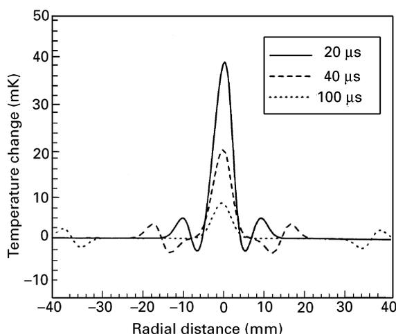
**Figure 3** Modelling of the gas temperature distribution as a function of the radial distance from the light excitation source. The diameter of the light beam was 6 mm and the pulse duration 20 ns. The three curves represent three different time delays after illumination.
