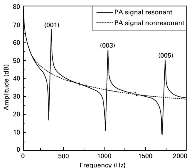
**Figure 6** Modelling of the frequency-dependent PA signal. The excited modes are the first (001), third (003) and fifth (005) longitudinal modes of the cavity. The dotted line shows the nonresonant contribution.
