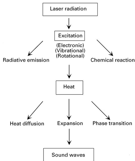
**Figure 1** Elementary processes occurring during PA signal generation. The absorbed photon energy is partly transformed into heat and acoustic energy.
