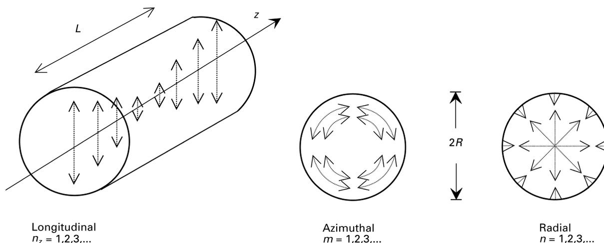
**Figure 5** Schematic representation of the longitudinal, azimuthal and radial acoustic modes in a cylindrical resonator.
