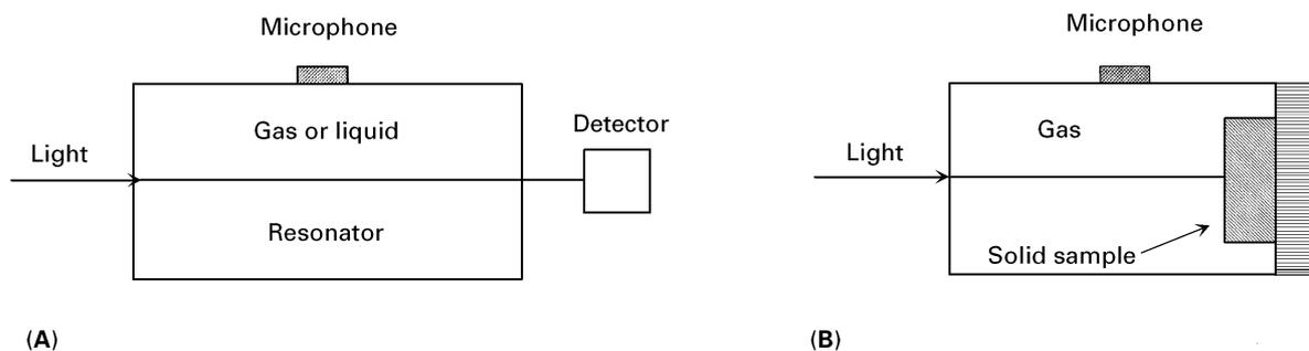
**Figure 4** PA setups for monitoring the PA signal with a microphone in a resonator: (A) gas or liquid, (B) solid sample in a gas microphone cell.
