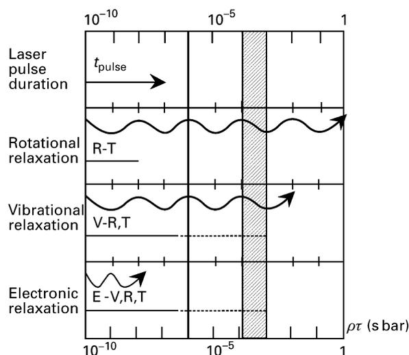
**Figure 2** Timescales for the radiative emission and relaxation processes. The shaded area indicates the typical response time of a PA resonator equipped with a microphone. The thick line represents the acoustic transit time. The wavy lines depict the radiative emission and the horizontal lines the range of relaxation processes characterized by the relaxation time  $\tau$ .
