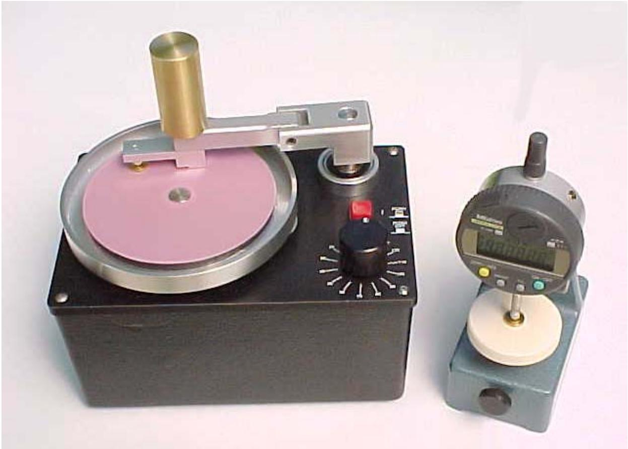
Figure 17. MTEC MicroLap equipment for removal of several micrometer increments of material from layered or gradient materials allowing chemical species profiles to be determined to arbitrary depths.
